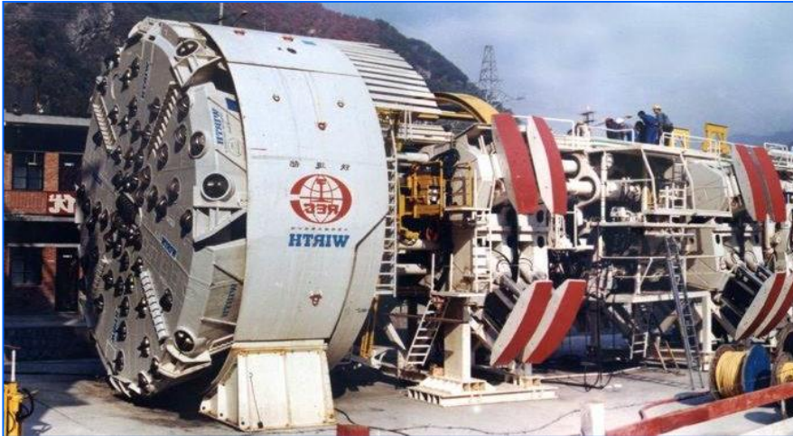
The TBM for the Xikang Qinling Tunnel, China
