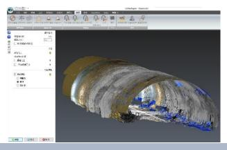
3D laser scan technology of tunnel section
